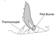
Figure 20 - Incorrect Pilot Flame Pattern
